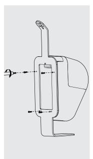
Attach the printer to the Bracket using M3x10mm Screws and T10 driver bit
