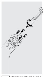
Remove Neck-Ring using T20 driver bit and Socket Driver
