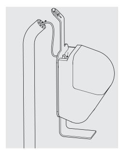
Feed power cable through Bracket and plug into Printer
