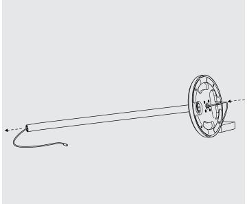
Feed the printer's power cable through the Floorstanding Pole  $\,$
